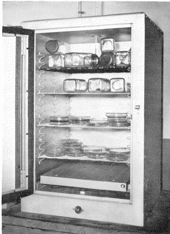
Incubation chamber containing Petri dishes and jars for testing materials in Federal Telecommunication Laboratories at New York.
